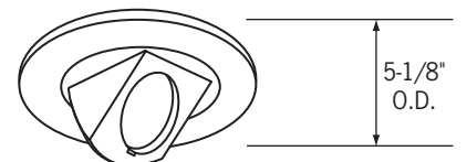
CTR1624G- (B, P) Fully Adjustable Square in Round, Select Finish 87° vertical and 359° rotation adjustment. Die-cast aluminum construction. Front access, spring latch lamp retainer ring. 47mm lens. Depth from ceiling: 2-1/2"
