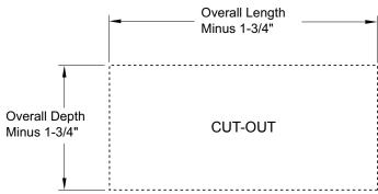
EXAMPLE: A DI-DP12X24 which measures 12" x 24" would require a cut-out size of 10-1/4" x 22-1/4"
